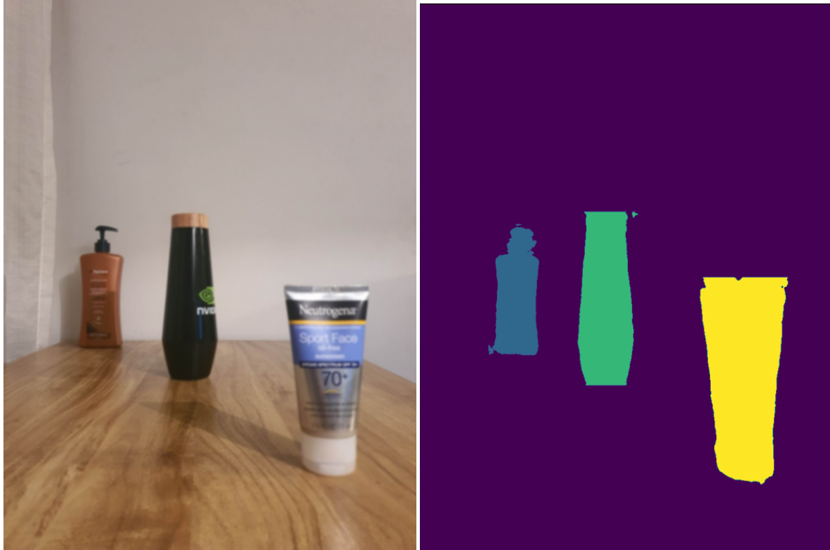
Figure 1. (Left) Image shows the input image, (Right) Image shows the depth map of the scene only for regions of interests. The different color indicate the depths of each of the regions.
