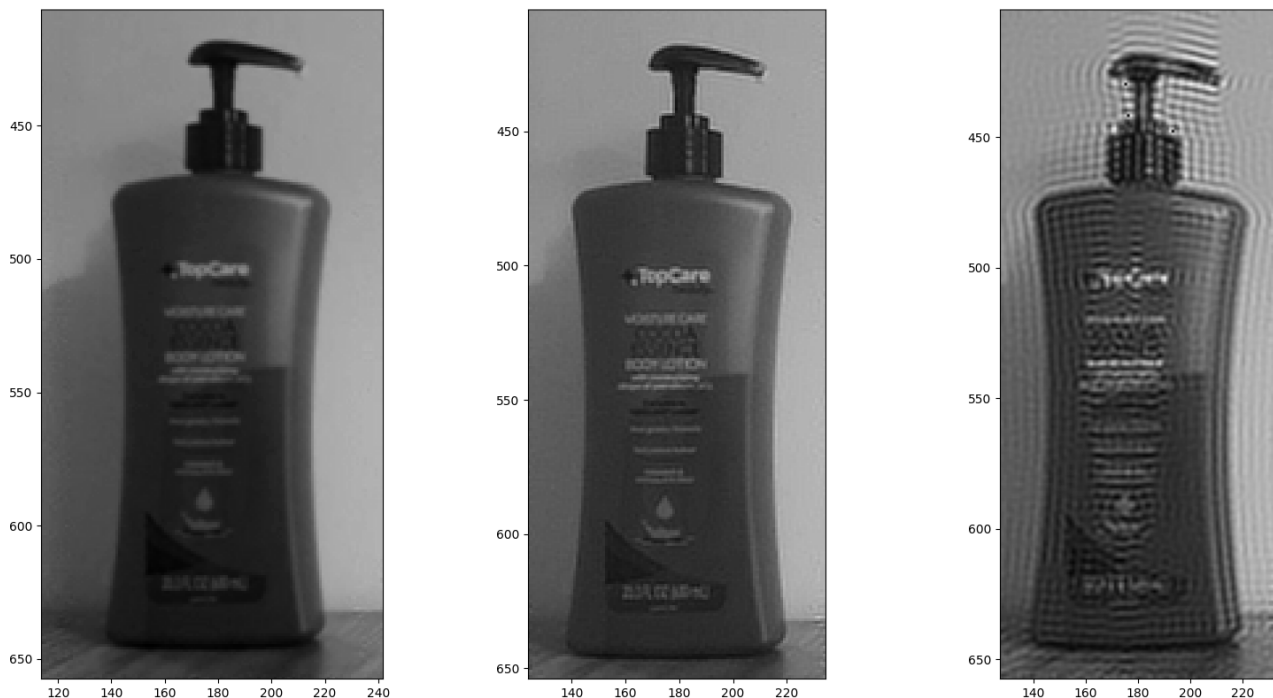
Figure 4. Figure shows the deconvolved image using kernels at different scales. When an incorrect kernel is used to deconvolve it produces artifacts.
